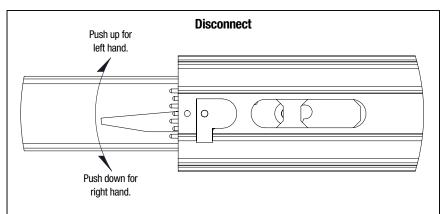
To disconnect drawer member, first extend the slide fully then lift up left hand slide disconnect lever and push down the right hand slide disconnect lever and pull drawer out.
